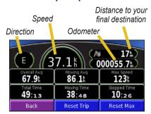
Touch **Reset Trip** to reset all information on the Trip Computer. To reset the maximum speed, touch **Reset Max**.
